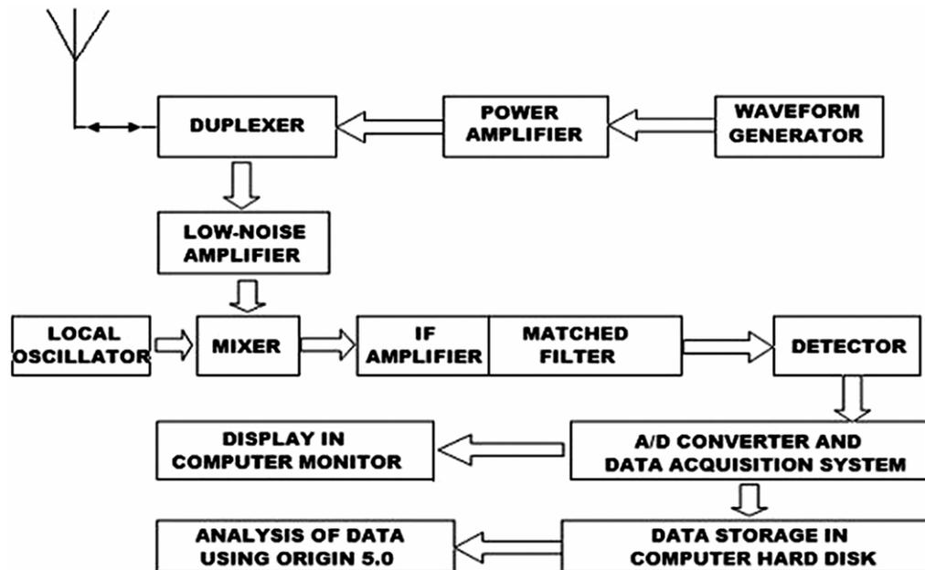
Fig. 1 — Schematic diagram of ELF-VLF receiver at Mirik
