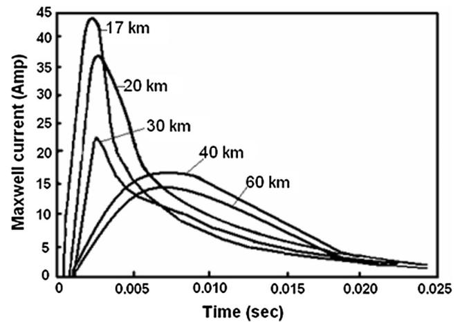
Fig. 3. Variation of Maxwell current  $(J)_{\text{Maxwell}}$  at different altitudes within the isotropic region. Time to reach currents a maximum is higher for higher altitudes which are marked in the plot. Five different altitudes above the upper boundary of the electrified cloud are chosen for computation.
