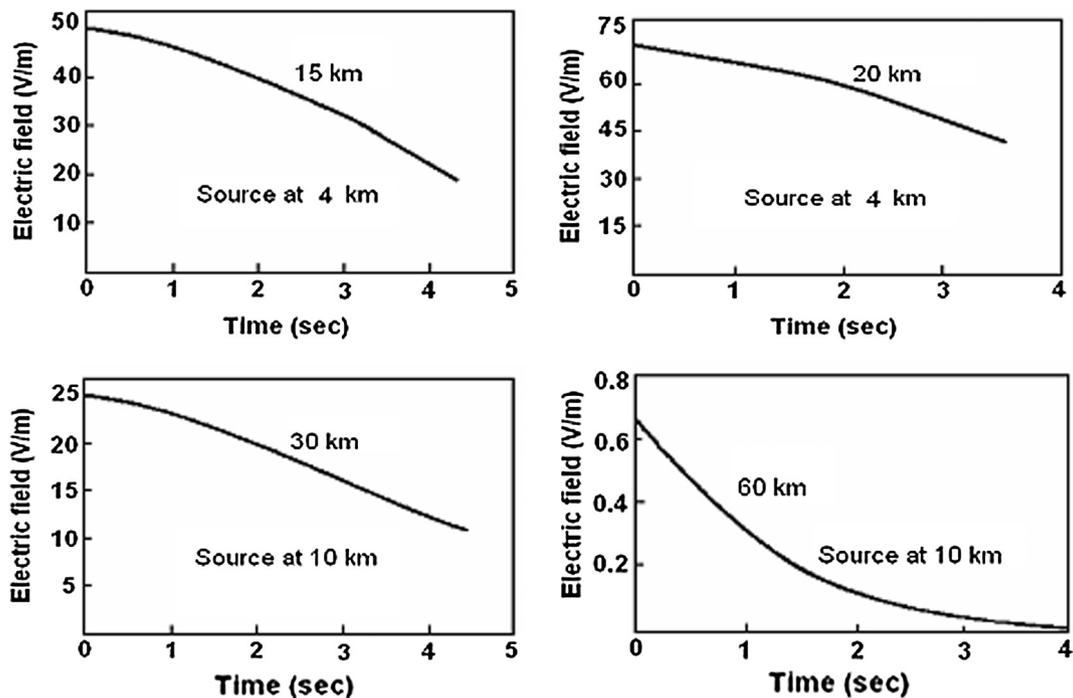
Fig. 4. Variations of electric fields at Kolkata (22.56°N, 88.5°E) Source heights are chosen at 4 km (near lower boundary of electrified cloud charge) and another at 10 km (near upper boundary of electrified cloud charge). Fields are computed in isotropic region. Maximum values are 48, 66, 24 and 0.65 V/m respectively.
