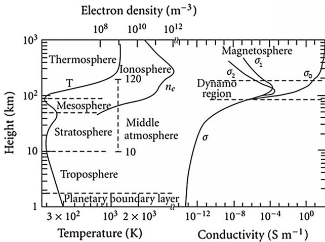
Fig. 2. Atmospheric electric conductivity, temperature and electron number density profile (Singh et al., 2004).
