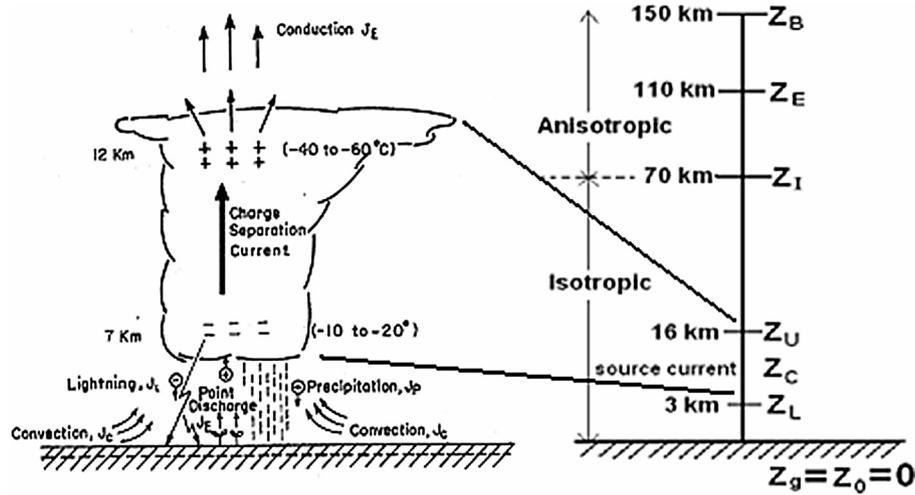
Fig. 1. Different current parameters involved within the distribution in cloud charge along with the schematic locations of various zones of the upper atmospheric region above the surface of the Earth. Discontinuity of longitudinal conductivity occurs at  $z = z_L$  and  $z = z_U$ .
