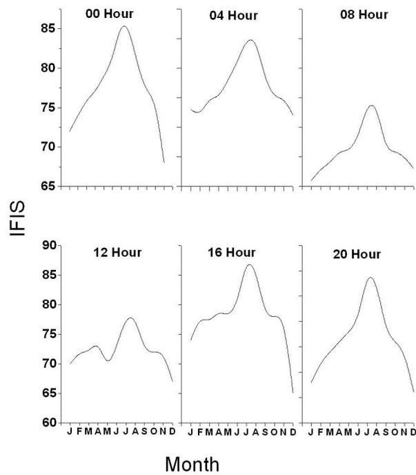
Figure 3. Monthly variation of IFIS at various hours of the day. The ordinate represents IFIS in terms of induced emf at the antenna in dB above  $1 \mu\text{V}$ .
