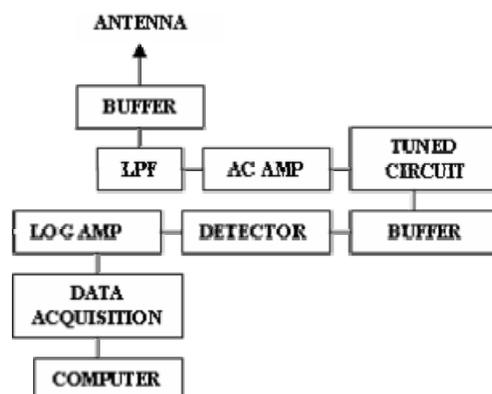
Figure 1. Block diagram of the receiver to record IFIS at 21.5 kHz.
