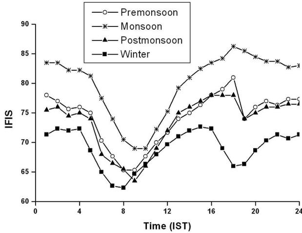
Figure 5. Diurnal variation of IFIS for various seasons. The ordinate represents the value in terms of induced voltage at the antenna in dB above  $1 \mu V$ .
