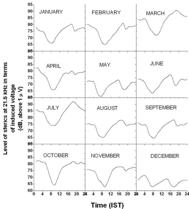
Figure 2. Diurnal variation of Integrated Field Intensity of Sferics at 21.5 kHz for various months. The ordinate represents the value in terms of induced voltage at the antenna in dB above 1  $\mu V$ .
