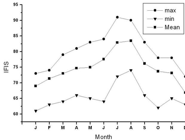
Figure 4. Graph showing the monthly variation of average level, maximum level and minimum level of IFIS of a day. The ordinate represents IFIS in terms of induced emf at the antenna in dB above  $1 \mu\text{V}$ .
