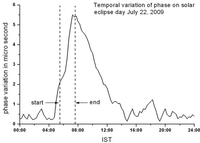
Figure 4. Retardation of phase of 19.8 kHz subionospheric signal in the propagation path as measured from Kolkata is shown.
