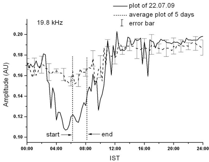
Figure 2. It depicts the amplitude variation of 19.8 kHz sub-ionspheric signal (continuous line curve) along with its averaged value for the adjacent 5 days (dotted line curve). The standard deviations from the average value are shown by error bars.
