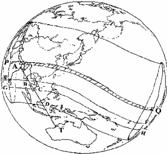
Figure 1. The detail of the eclipse path and propagation path are depicted. **PQ** is the path of totality. The lines **EF** and **GH** represent the occurrence of 60% and 40% of the totality during maximum phase. **T** is the transmitting centre, **A** is the receiving centre and **TA** shows the propagation path.
