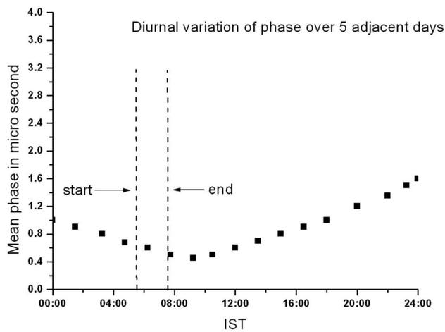
Figure 3. The variations of the mean phase averaged over 5 adjacent days of the day of occurrence of the eclipse at every 15 minutes interval are presented. 3 adjacent days prior to and 2 adjacent days after the solar eclipse.
