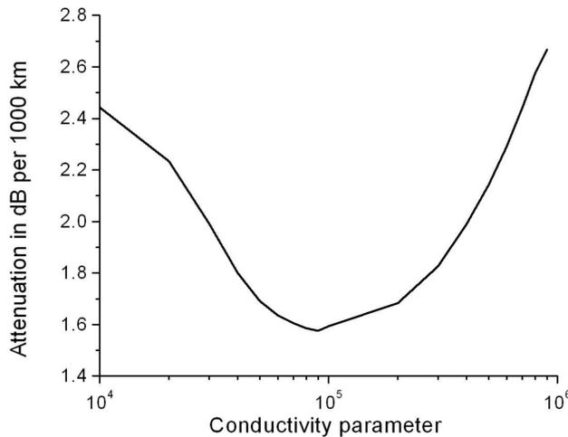
Figure 5. Variation of attenuation (in dB per 1000 km) with conductivity parameter according to waveguide mode theory at 19.8 kHz.
