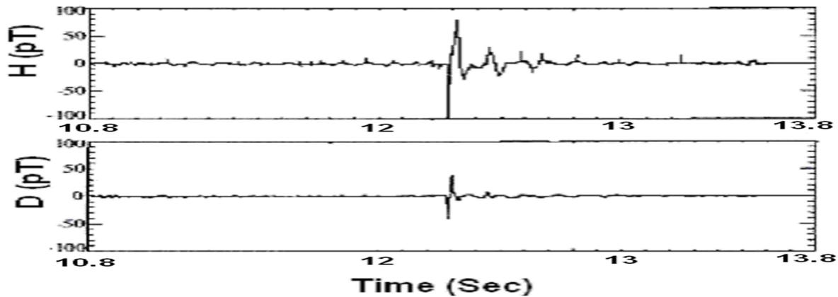
Figure 3. Plots of H (North-South) and D (East-West) components of ELF bursts recorded near Bay-of-Bengal on December 24, 2009 between 04:04:10.8 and 04:04:13.8 hrs UT. The time difference between the direct and antipodal pulses is about 130 msec
