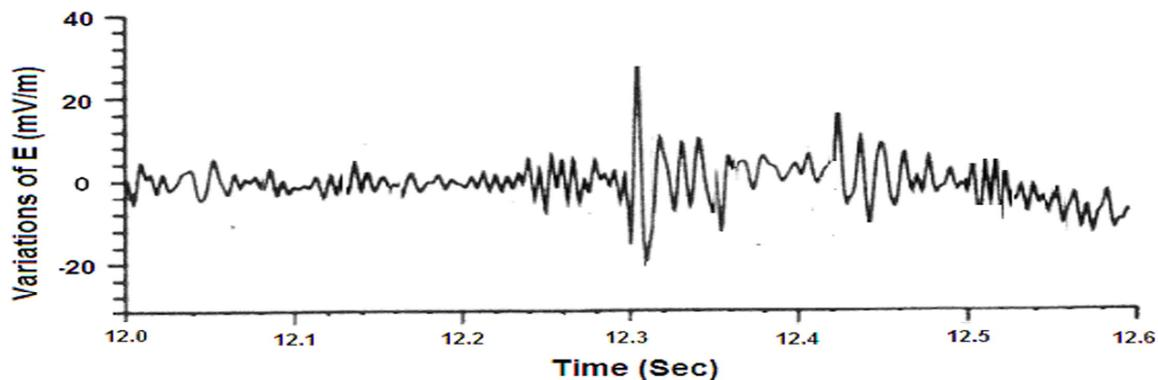
Figure 4. Plots of Electric field component of ELF bursts recorded by ball antenna near Bay-of-Bengal on December 24, 2009 between 04:04:12.0 and 04:04:12.6 hrs UT
