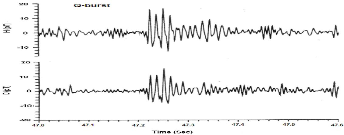
Figure 1. Plots of H (North-South) and D (East-West) components ELF data recorded near Bay-of-Bengal on July 4, 2000 between 06:32:47.0 and 06:32:47.6 hrs UT
