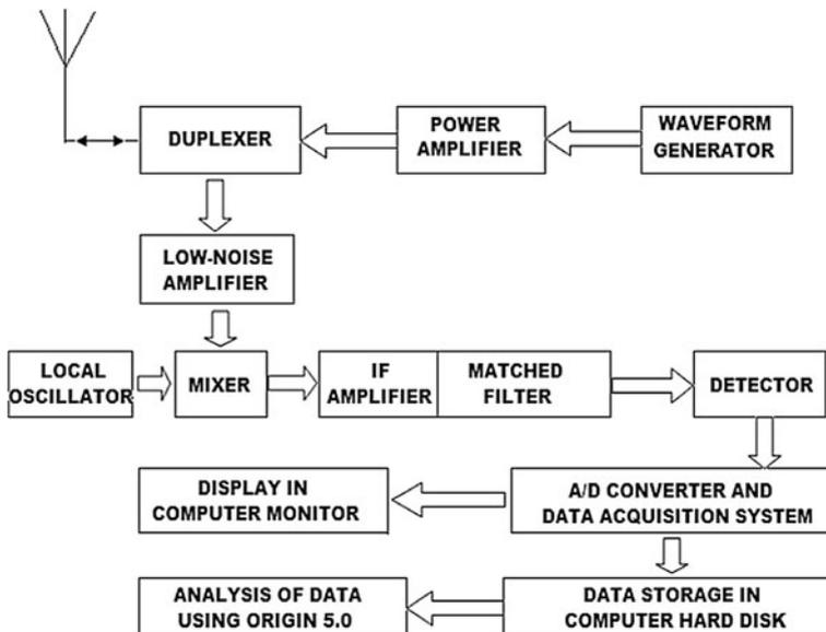
**Fig. 1** Block diagram of the receiving system
