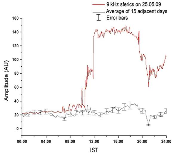
Figure 3. Temporal variation of sferics at 9 kHz on May 25, 2009 are shown by the red coloured curve while the average of adjacent 15 days of occurrence of AILA is given by the black coloured curve. The standard deviations are shown by error bars.
