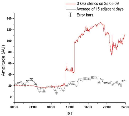
Figure 2. Temporal variation of sferics at 3 kHz on May 25, 2009 are shown by the red coloured curve. The average of adjacent 15 days of occurrence of AILA is shown by the black coloured curve. The standard deviations are shown by error bars.
