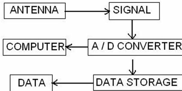
Figure 1. Block diagram of VLF measurement system
