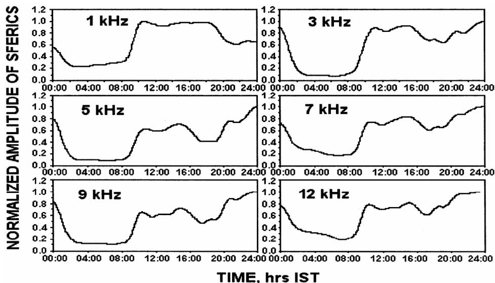
Fig. 2 — Diurnal variation of sferics in winter season (November and December 2004, and January and February, 2005) at various frequencies [The strength of the sferics has been shown in terms of the normalized value of induced voltage at the antenna]
