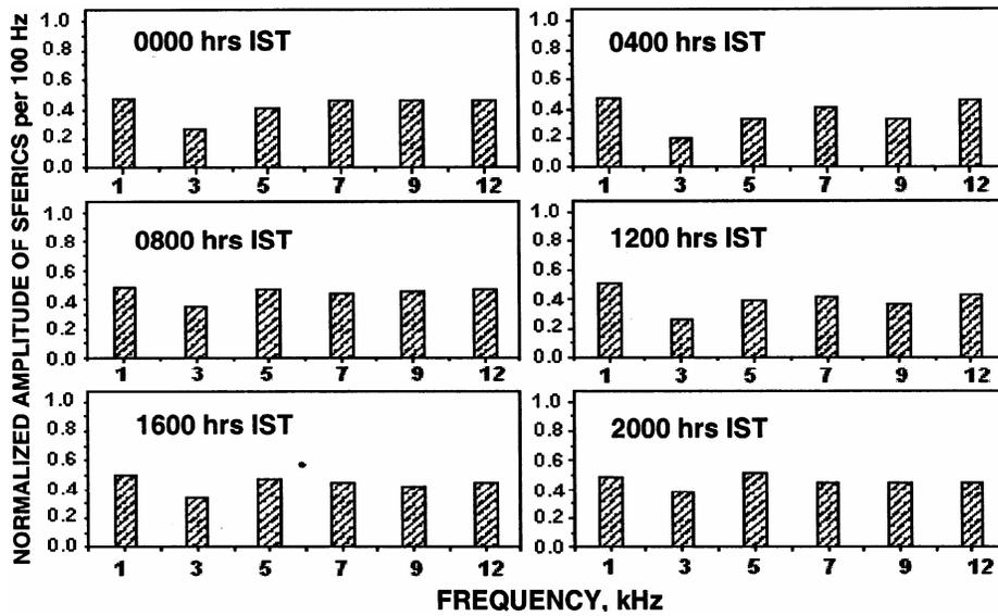
Fig. 3 — Sferics spectrum at various times in rainy days
