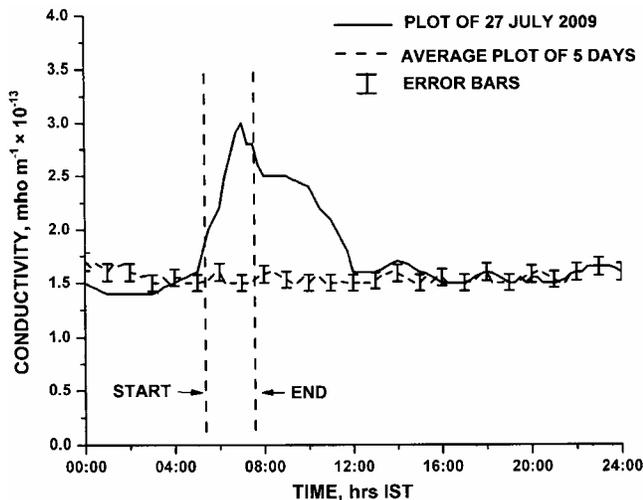
Fig. 4 — Temporal variation of ground level conductivity at Kolkata presented by the continuous line curve during solar eclipse on 22 July 2009 [dotted line curve represents averaged value over adjacent five days; standard deviation from the average are shown by error bars]
