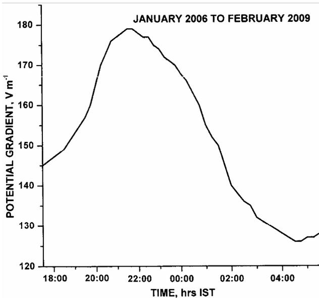
Fig. 3 — Night time variation of atmospheric vertical electric potential gradient averaged over 90 fair-weather days during January 2006 - February 2009
