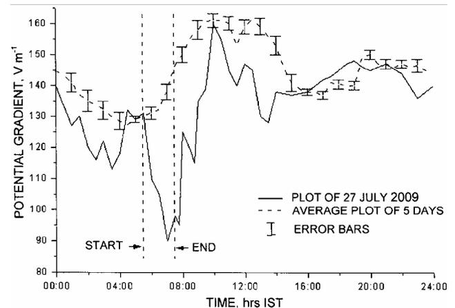
Fig. 2 — Temporal variation of atmospheric vertical electric potential gradient over Kolkata presented by the continuous line curve during solar eclipse on 22 July 2009 [dotted line indicates average value over adjacent five days; standard deviation from the average are shown by error bars]
